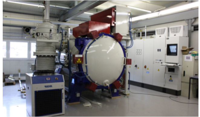
Vacuum brazing furnace at DAU
